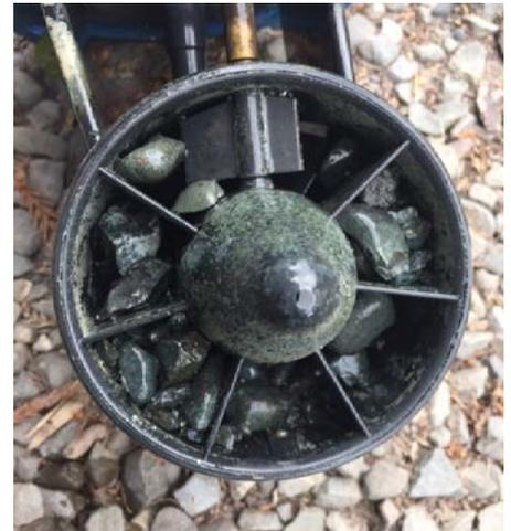
A maintenance 'what not to do'... this meter was so full of stones it didn't work. A stone trap is needed.
