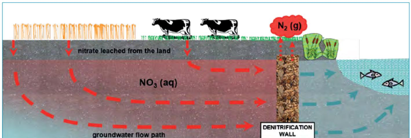
A concept diagram illustrating nitrate removal via a denitrification wall. Carbon substrate within the wall provides a food source for denitrifying microorganisms that respire nitrate. Any nitrate in groundwater passing through the wall is converted to harmless di-nitrogen gas ( $N_2$ ).
