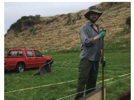
Brian Levine, PhD student at Massey University, installing a V-notch weir to measure storm water flows at a detainment bund site in the Lake Rotorua catchment.
